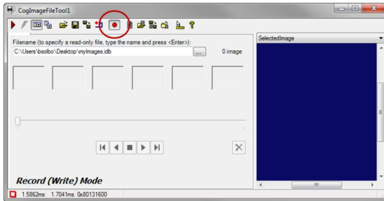
Write Mode is designated by pressing the red circle which is the record button. Now every time an new image comes into the toolgroup, it will save the image into the database.
